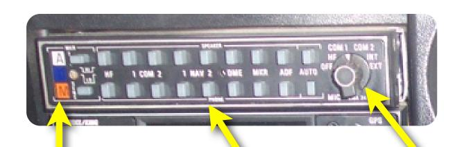
The ILS Marker Beacon lights tell an instrument pilot where they're at on final approach.
