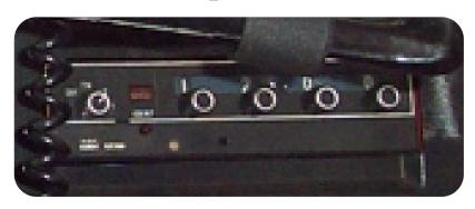
This box sends the dialed in 4-digit number to the RADAR facility to identify our airplane. It will normally be set to 1200 if we're not getting any RADAR services from ATC. The light will flash every time we send the number.
