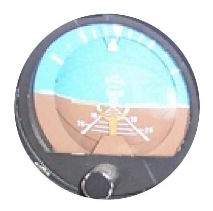
This shows the angle of climbs and descents and the angle of bank during turns. This gauge should look like the view out the front window - blue corresponds to sky, brown corresponds to ground.
