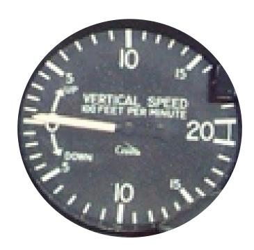
This shows how fast we're ascending or descending. If the needle is pointing at the 5 on the top half, we're ascending at 500 feet per minute. If the needle points to 7 on the bottom half, we're descending at 700 feet per minute
