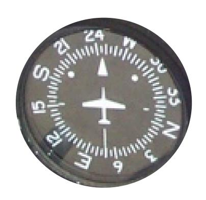
This is similar to a compass, but instead of using a magnet to determine direction, it uses a gyroscope. Because the gyro drifts a bit, I'll be resetting it to match the magnetic compass periodically.
