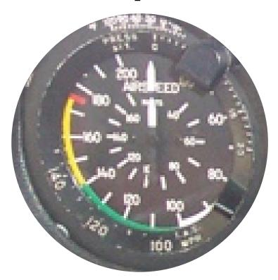
This shows how fast we're traveling through the air. There are two scales on the gauge: one is nautical MPH (knots), and one is statute MPH (the same you use in your car)
